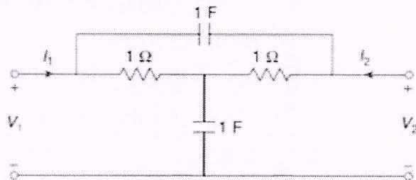
20 (a) Find open circuit impedance parameters of the given network. (7)
