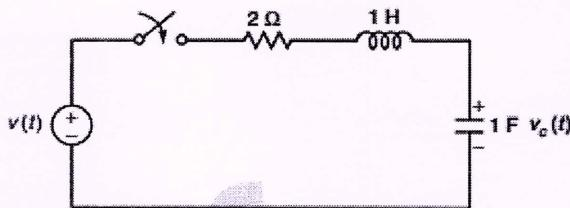
(b) The network was initially in steady state with the switch in position a. The switch is moved from a to b, at  $t = 0$ . Find  $v(t)$  for  $t > 0$ . (6)
