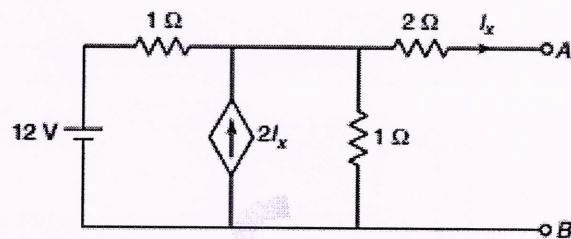
(b) Determine the current through  $1\Omega$  for the network given below using (7) superposition theorem.
