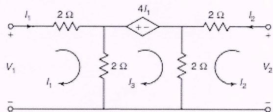
(b) Derive the conditions for reciprocity and symmetry for ABCD parameters. (7)
