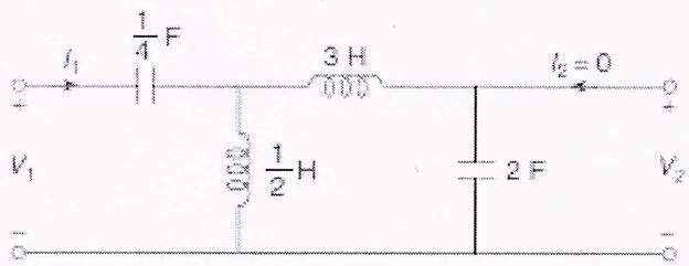
18 (a) Find the network functions  $\frac{V_1}{I_1}$ ,  $\frac{V_2}{V_1}$  and  $\frac{V_2}{I_1}$ , for the network given below. (6)
