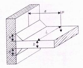
b) A bracket shown in figure carries a load of 10 KN. Find the size of the weld if the (10) allowable shear stress is not to exceed 80 MPa.
