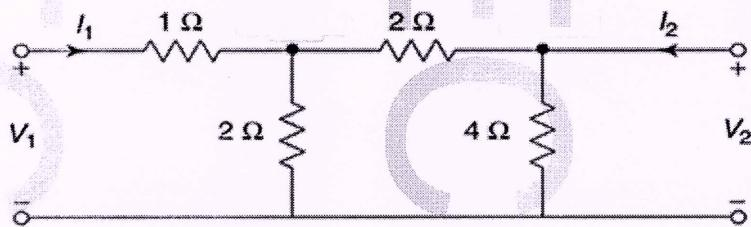
16 a) Show that when two port networks are connected in parallel, the resultant Y matrix is the sum of Y matrices of each individual network. CO4 (5)
