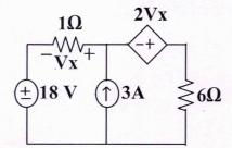
(b). Using superposition theorem determine Vx. Also determine the power (5) delivered by Vx.
