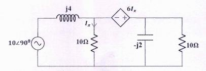
12 (a) Determine the voltages  $V_x$  and  $V_y$  using node analysis
