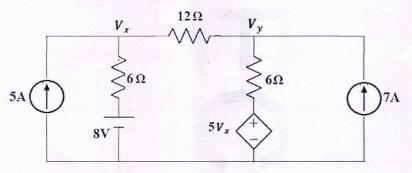
(b) Evaluate the current  $I_c$  in the following network using mesh analysis. (6)
