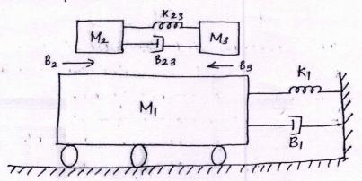
13 b) Write the equations of motion in S-domain for the system given in figure below.
