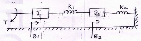
14 b) Write the differential equations governing the mechanical rotational systems shown in figure.obtain the transfer function of the system.
