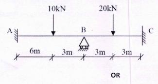
16 a) Analyse the frame shown below using stiffness method and draw the BMD (14)
