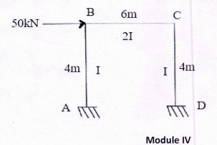
17 a) Analyse the continuous beam shown in figure by direct stiffness method and draw (14) the Bending moment diagram.
