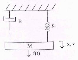
12 a) Find the differential equation governing the mechanical system shown in fig. 10 Obtain the corresponding Force-Voltage analogous circuit.
