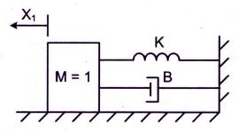
b) Determine the condition for the asymptotic stability of the system described by (6) the state equation given below using Lyapunov method
