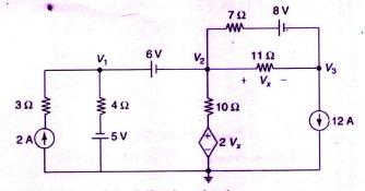
b. Find the node voltages of the following circuit.
