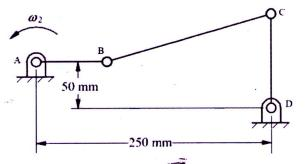
For the four-bar mechanism shown in figure, link AB is rotating CCW at the rate of 2 rad/s (constant). The link AB is horizontal and link CD is vertical. Given AB = 75 mm, CD = 100 mm. Determine the angular velocity of BC and CD.
