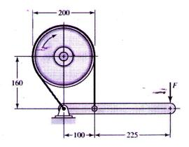
b) The block-type hand brake shown in the figure (with dimensions in cm) has a face (6) width of 12.5 mm and a mean coefficient of friction of 0.25. For an estimated actuating force of 900 N, find the maximum pressure on the shoe and find the braking torque
