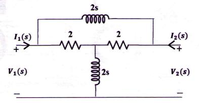
20 Two identical sections of the following network are connected in series-parallel (14) combination. Determine the hybrid parameters
