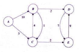
Write Kruskal's algorithm for minimum spanning tree (MST). Apply this (10) algorithm to find a MST of the below graph.
