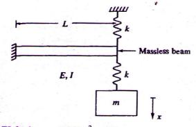
Take L = 3m. EI for beam = 27  $\text{Nm}^2$ , stiffness for each spring, k = 3 N/m and mass m= 3 kg
