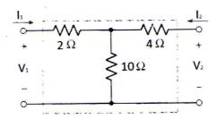
6 Check for symmetry and reciprocity of a two port network in z parameter (5) representation shown in figure
