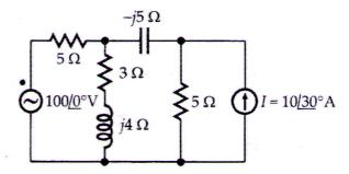
10 a) Determine the Norton equivalent circuit for the network shown in figure
