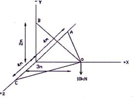
11 a) Find the reactions at the supports A(hinged) and B (roller).
