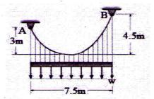
8 a) A three-hinged parabolic arch is loaded as shown in figure. Calculate the location and magnitude of maximum bending moment in the arch. Draw bending moment diagram.
