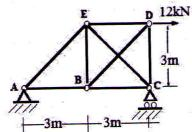
Analyse the beam shown using consistent deformation method and draw the SFD (15) and BMD
