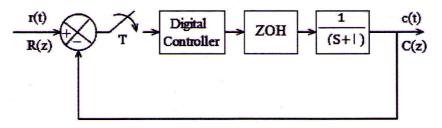
Design a digital controller for the system shown in figure using root locus method to meet the following specifications.
