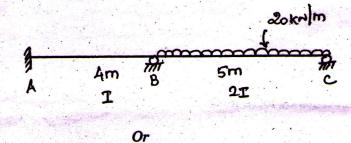
16. Analyse the given frame by direct stiffness method :
