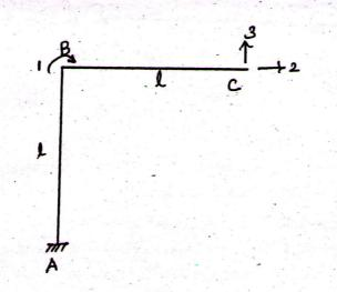
3. Determine stiffness matrix of a beam as shown in figure :
