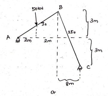
12. Analyse the given truss by force method :
