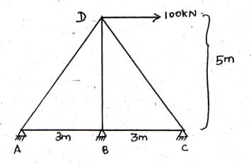
13. Analyse the given element by displacement method. Draw the Bending moment diagram :
