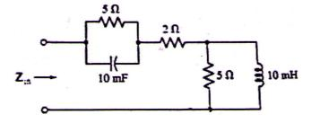
8. a. Find yparameters for the two-port network shown in figure.
