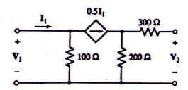
b. Calculate h parameters for the two-port network shown in figure.
