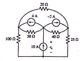
b. Find the Thevenin equivalent of the network shown in figure. What power would be delivered to a load of 100 ohms at a and b? (6)
