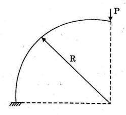
13. (a) Analyse the beam using method of consistent deformation and determine the reaction components and draw shear force and bending moment diagram.
