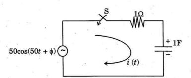
13. (a) Find the transfer functions  $G_{21}(s)$ ,  $z_{21}(s)$  and driving point impedance  $z_{11}(s)$  of the following circuit.
