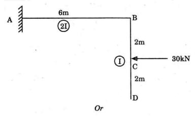
(b) Analyse the structure shown in fig. by strain energy method. Sketch the bending moment diagram.
