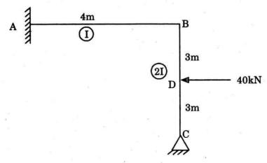
13. (a) Determine the reaction components and draw the shear force and bending moment diagram for the given beam, if the support A, B, C and D settles by 20 mm, 40 mm, 60 mm and 80 mm. consider  $E - 2 \times 10^6$  N/mm<sup>2</sup>, and  $I - 3 \times 10^6$  mm<sup>4</sup>.
