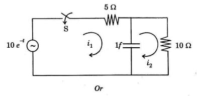
(b) For the following circuit, find the current when the switch is moved from position 1 to position 2 at t = 0. The switch has been in position for a long time to get steady state values.
