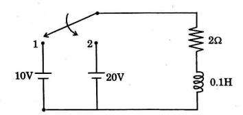
13. (a) Draw the pole zero diagram for the given network function I (s) and hence obtain i(t)
