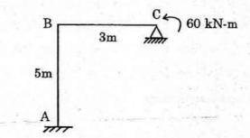
III. (a) Generate the stiffness matrix for the following beam with co-ordinates as shown.
