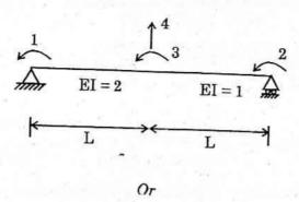
(b) Find the displacements over supports and member end forces for the beam shown below. Use stiffness approach. (L = 4m).
